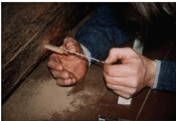
Cores of timbers reveal tree-ring patterns making it possible to date historic structures. Image: Lamont-Doherty Earth Observatory Columbia University Earth Institute
